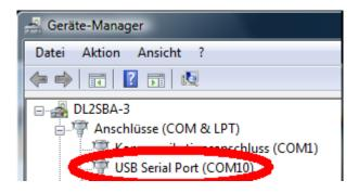
Remember the name of the newly added COM-port - here COM10. It will be later used inside vna/J application to select the correct COM-Port for the miniVNA.
